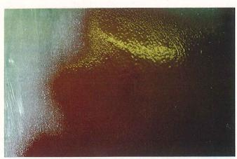
ABOVE ▲ The specs called for Polyshield HT, an aromatic polyurea, which can change color when exposed to UV rays. So, the crew used a formulation of Polyshield HT in a terra cotta color with a high pigment load and a UV enhancer to reduce color fading.
